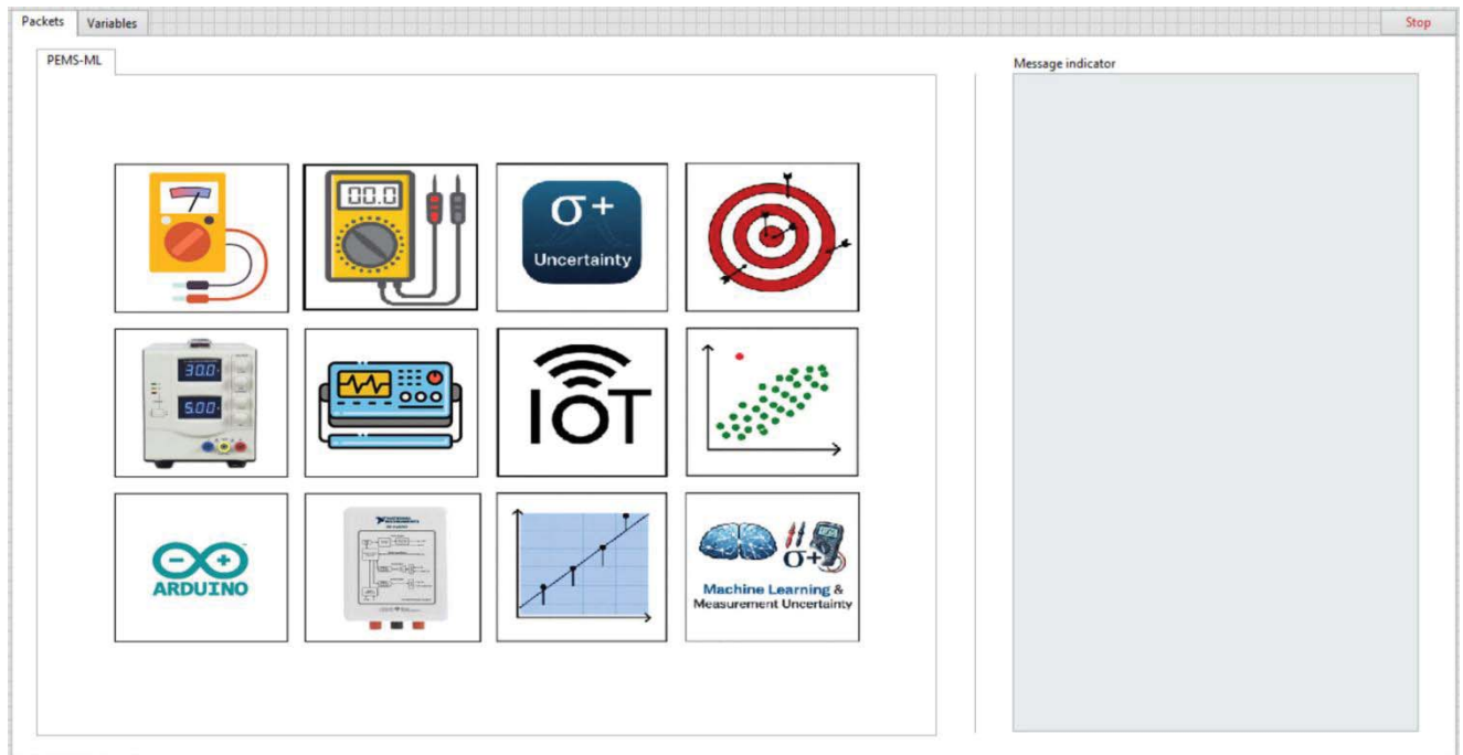
Fig. 1. Front panel of the LabVIEW-based virtual framework, showing the instrument-centric Packets tab for launching specialised virtual instruments, and the Variables tab for visualising data exchanged through software-defined virtual channels.
